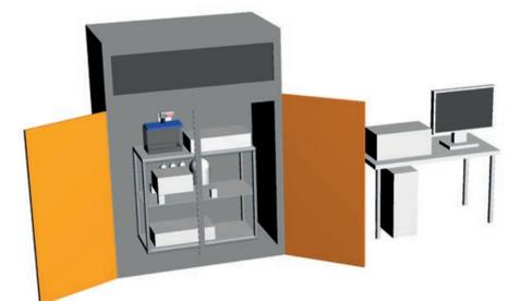
Illustration of the modular test-bed with the breadboard model inserted into an incubator controlling temperature and relative humidity. Data acquisition and remote control capabilities are offered by an external computer which serves as a user interface for the breadboard system. Illustration: DTM
